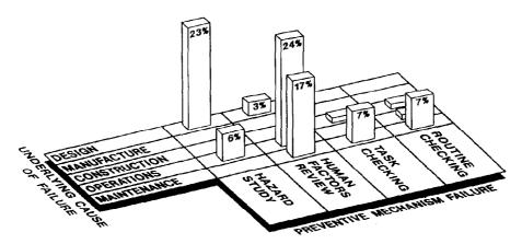
Figure 1 Analysis of accident data: Major Accident Reporting System (MARS)11
