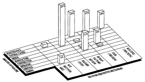
Figure 1 Underlying causes of pipework failures4
